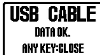
The following screen will appear if a cable that does not support data transfer has been used. Replace the cable with one that supports data transfer.
