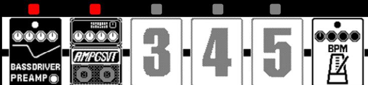
The diagram shows a pedalboard with the following components from left to right: a Bass Driver Preamp pedal, an Ampsim pedal, three delay pedals labeled 3, 4, and 5, and a BPM pedal. Above the pedals are five indicator lights: the first two are red, and the last three are grey.
