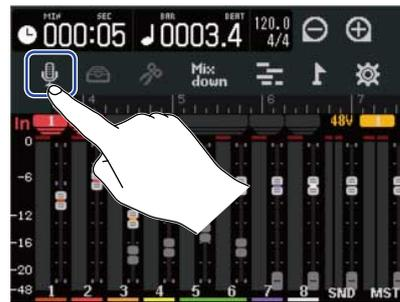
This opens the Input Routing Screen.
