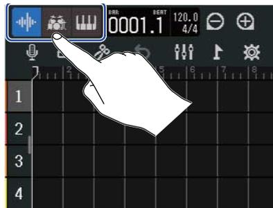
When set as a rhythm or synthesizer track, the track number will be replaced with a rhythm or synthesizer track icon.
