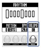
This adjusts the volume of the rhythm in the memory. To adjust the overall volume of the MS-90LP+ , see "Adjusting the overall output level (OUTPUT VOLUME)".
