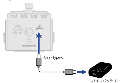
When a portable battery is connected, the MS-90LP+ will power on.
