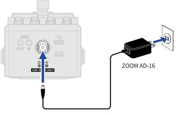
When an AC adapter is connected, the MS-90LP+ will power on.
