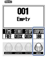
This adjusts the volume of the loop in the memory. To adjust the overall volume of the MS-90LP+, see "Adjusting the overall output level (OUTPUT VOLUME)".
