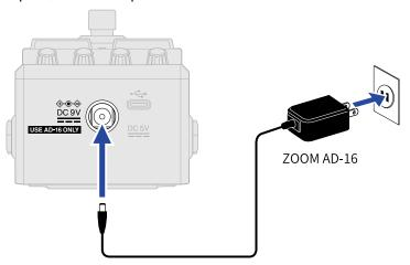
When the AC adapter is connected, the MS-50G+ will power on.
