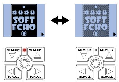
The On/Off indicator lights when the effect is on.
