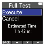
The result of the test will be shown when it completes. If the access rate MAX reaches 100%, the card will fail (NG).
