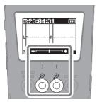
The M2 uses 32-bit float format, which can record with the same resolution for any volume level, so adjusting the recording level is unnecessary. During playback, the top and bottom edges of the waveform screen are the highest volume levels.
