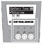
Set the type of battery used correctly so that the amount of remaining battery charge can be shown accurately.
