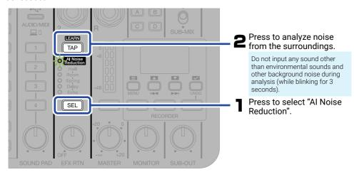
Al Noise Reduction is applied to signals sent to the MASTER. It does not affect the recording data for each channel.
