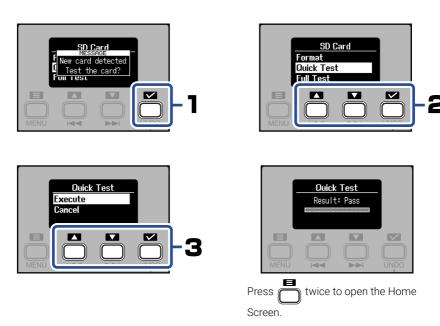
A full test will check the entire microSD card, so the amount of time required depends on its capacity (about 2.5 hours for 64 GB).
