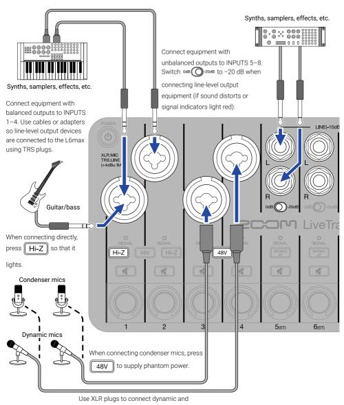
Do not supply phantom power to devices that are not compatible with it. Doing so could damage those devices.
