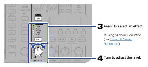
• The tempo used for Delay and Echo can be set by repeatedly pressing TAP at a regular interval.
