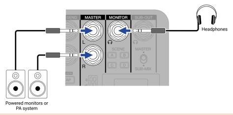
To prevent noise and malfunction, connect powered monitors before turning the power on.
