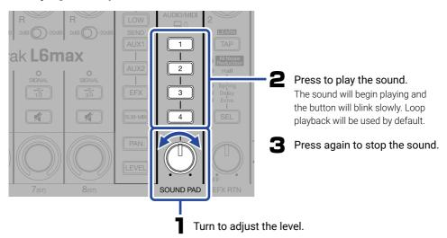
Audio files assigned to sound pads can be removed and changed from the Menu Screen. In addition, their play
