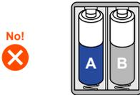
Do not mix batteries of different types or made by different manufacturers.
