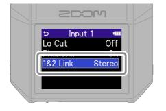
When stereo-linked, tracks are recorded as a stereo file with the odd-numbered track on L and the even-numbered track on R.
