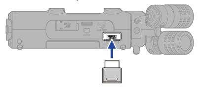
2. Slide the (POWER/HOLD) switch toward (in the direction of the INPUT 1 and 2 jacks) to turn on the power.
