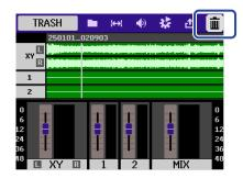
2. Use the (selection) dial to select "Execute" and press the (ENTER) button. This moves the file being played to the trash. (→ H5studio folder and file structure)
