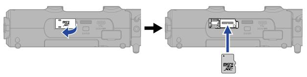
To remove a microSD card, push it further into the slot and then pull it out.
