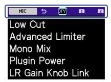
3. Use the (selection) dial to select "LR Gain Knob Link" or "1&2 Gain Knob Link" and press the (ENTER) button.
