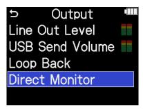
3. Use the (selection) dial to select "On" or "Off" and press the (ENTER) button. Selecting "On" turns on the direct monitoring function.
