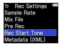
3. Use the (selection) dial to select the recording start tone level and press the button to confirm. (ENTER)
