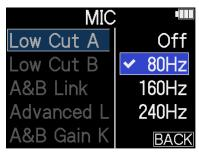
Lo Cut can be set to OFF, 80 Hz, 160 Hz or 240 Hz.
