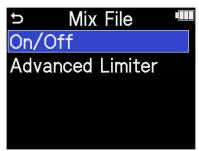
**4.** Use the (selection) dial to select "On" or "Off" and press the ENTER (ENTER) button to confirm.
