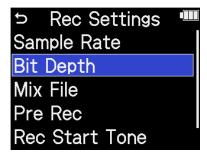
3. Use the (selection) dial to select the bit depth and press the (ENTER) button to confirm.
