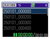
Use the  $\bigcirc$  (selection) dial to select setting items and press the  $\bigcirc$  (ENTER) button to conduct operations. ( $\rightarrow$  File List Screen)
