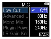
Low Cut can be set to Off, 80 Hz, 160 Hz or 240 Hz.
