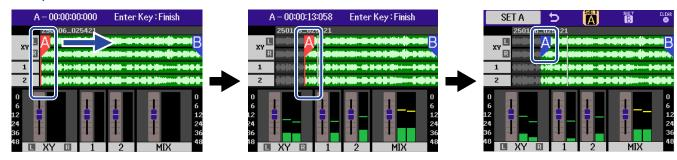
Pressing the  $\bigcap_{\text{ENTER}}$  (ENTER) button confirms the A point and makes the A marker become blue.
