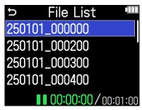
2. Use the (selection) dial to select a file and press the (ENTER) button. A menu bar that enables operations on the selected file will appear.
