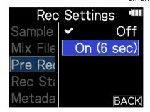
The amount of time that can be pre-recorded when this is set to "On" depends on the sample rate setting ( $\rightarrow$  Setting the sample rate).
