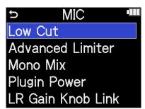
**4.** Use the (selection) dial to select the cut frequency and press the (ENTER) button.
