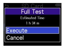
The result of the test will be shown when it completes. If Access Rate Max. reaches 100%, the card will fail (NG).
