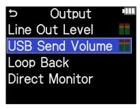
3. Use the (selection) dial to adjust the USB output level and press the (ENTER) button. The output level meters can be checked while adjusting.
