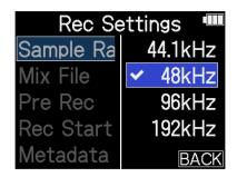
The following sample rates can be selected. 44.1 kHz, 48 kHz, 96 kHz, 192 kHz
