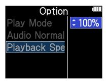
The following speeds can be selected. 50% (half speed), 75%, 100% (normal), 125%, 150%, 200% (double speed)
