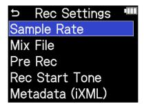
3. Use the (selection) dial to select the sample rate and press the (ENTER) button to confirm.
