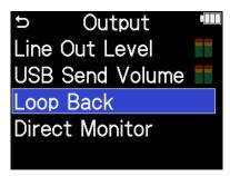
**3.** Use the (selection) dial to select "On" or "Off" and press the ENTER) button. Selecting "On" turns on the loopback function.
