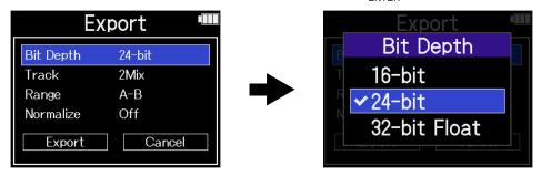
The following formats can be selected. 16-bit, 24-bit, 32-bit Float
