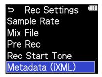
3. Use the (selection) dial to select "Write" or "Off" and press the (ENTER) button to confirm.
