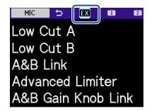
3. Use the \_\_\_\_\_ (selection) dial to select "Low Cut A" or "Low Cut B" and press the \_\_\_\_ (ENTER) button.
