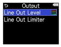
5. Use the (selection) dial to adjust the line output level and press the (ENTER) button. The output level meters can be checked while adjusting.
