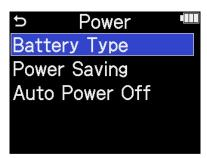
**4.** Use the (selection) dial to select the battery type and press the (ENTER) button.
