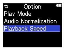
3. Use the  $\bigcirc$  (selection) dial to select the playback speed and press the  $\bigcirc$  (ENTER) button.
