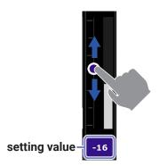
When the volume setting of a track is being adjusted, the setting value will be shown numerically instead of the track name.
