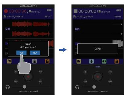
This will stop recording and move the file being recorded to the TRASH folder.
