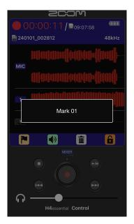
This will add a mark at the position of the current elapsed recording time. The playback position can be moved to a mark during playback.
