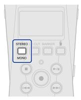
Pressing this switches between STEREO and MONO.
