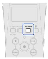
This will add a mark at the position of the current elapsed recording time.
