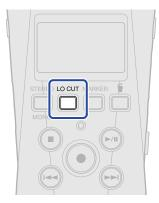
The cutoff frequency can be selected and set to OFF, 80 Hz, 160 Hz or 240 Hz.
