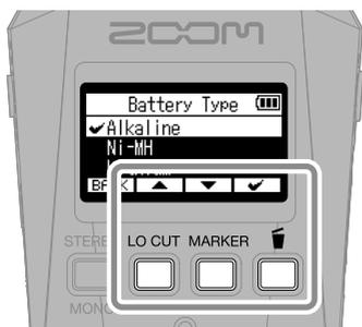
Set the type of battery used correctly so that the amount of remaining battery charge can be shown accurately.
