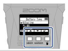
Set the type of battery used correctly so that the amount of remaining battery charge can be shown accurately.
