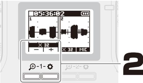
Use (/) to adjust the waveform display size.
