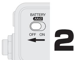
To use USB bus power, set the BATTERY switch to OFF.
