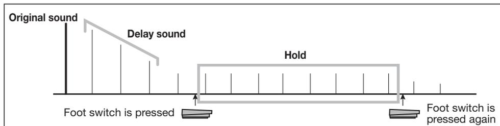
will activate hold, causing the current delay sound to be repeated (see illustration below). Pressing the foot switch once more cancels the hold condition, and the delay sound will decay normally.
