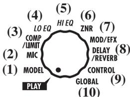
When you set the Module selector to a position other than "PLAY", the A2 switches to edit mode, and the effect type currently selected for the respective module is shown. In edit mode, a dot appears in the bottom right of the display.
