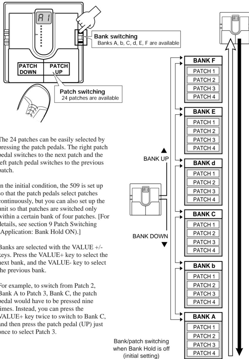
The 24 patches can be easily selected by pressing the patch pedals. The right patch pedal switches to the next patch and the left patch pedal switches to the previous patch.
