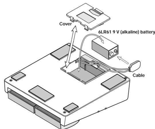
1. Turn the 504 upside down and open the cover of the battery compartment. (Push the catch to unlock the cover, then lift it up.)
