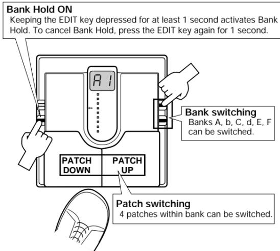
Bank/patch switching when Bank Hold is on
