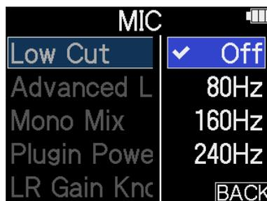
Low Cut can be set to Off, 80 Hz, 160 Hz or 240 Hz.
