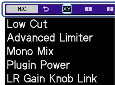
3. Use the
