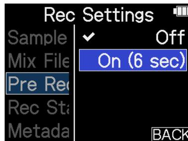
The amount of time that can be pre-recorded when this is set to "On" depends on the sample rate setting (→ [Setting the sample rate](#)).
