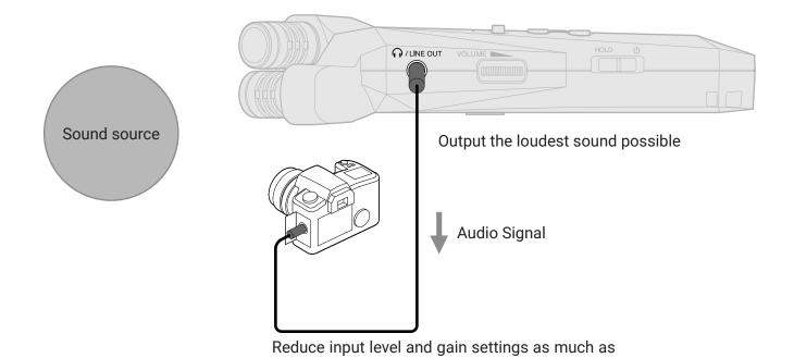
When setting the level, while observing the camera level meter, raise the output of the recorder keeping it just below the level that would cause the audio source being recorded to clip. Do not use the auto gain control function of the camera because doing so could increase the volume of noise.
