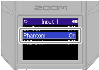
Turn on phantom power for inputs that have condenser mics connected.
