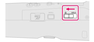
This turns the M2 power on and opens the Home Screen on the display.
