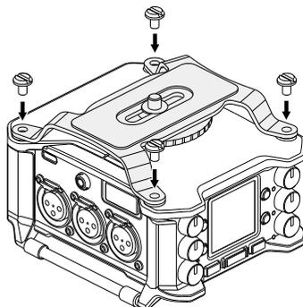
3. Attach the **F6** to a tripod, for example, and then attach the camera with the camera mount adapter screw.
