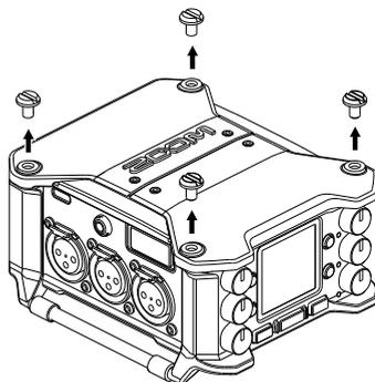
2. Align the screw positions of the camera mount adapter with those of the **F6**, and tighten the screws.
