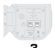
CH.1 CH.2 Press  $\bigcirc$ / $\bigcirc$  to light the channels that have mics connected to them.
